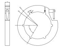
Coil stops are anchored to the body shaft using a latch and set the limit for positioning the coils. They can be for body shaft diameter of 150mm or any other custom measures
